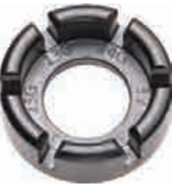
TB-5510 "O" spoke wrench •Forged with 8 grooves to adjust spoke tension for 9 G ~ 15 G nipples. •It is a very useful tool for DIY users.
