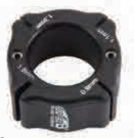
TB-5501 Aero spoke key •Steel core covered with nylon prevents the flat spokes turned when adjusting the nipple of spoke. •A ring design makes easier and more stable operation when wearing on the finger. •Fix Aero spoke, size: 0.9 / 1.1 / 1.3 / 1.9 mm.
