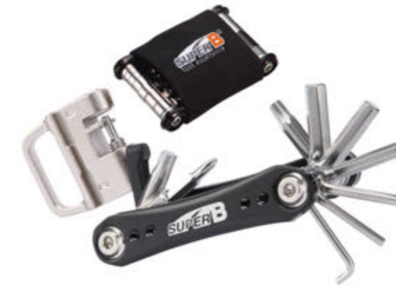
TB-FD20 18 in 1 folding tool • 2 / 2.5 / 3 / 4 / 5 / 6 / 8 mm hex key wrench. • Phillips 1 screwdriver, T25 / T30. • Tire lever x 2. • Pin holder. • W/ vinyl housing. • Chain rivet extractor with spoke wrench 3.2 / 3.5 / 3.3 / 3.5 mm. • One-piece forged bits are for superior durability.
