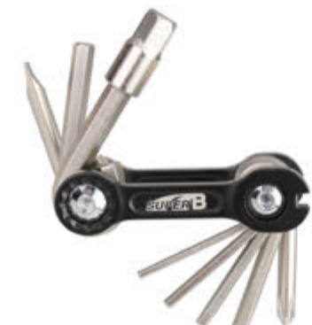
TB-9870 10 in 1 folding tool • 2 / 2.5 / 3 / 4 / 5 / 6 / 8 mm hex key wrench. • Spoke wrench 3.2 mm. • Phillips 2 and slotted 5 screwdrivers.
