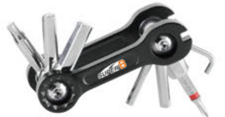
TB-9855 9 in 1 folding tool • 2 / 3 / 4 / 5 / 6 / 8 mm hex key wrench. • Spoke wrench 3.2 mm. • Phillips 1 screwdriver, T25. • One-piece forged bits are for superior durability.
