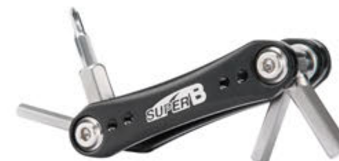
TB-FD10 7 in 1 folding tool • 4 / 5 / 6 / 8 mm hex key wrench. • Phillips 1 screwdriver. • Tire lever x 2. • One-piece forged bits are for superior durability.
