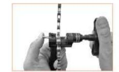
Push the pin guider to touch the pin chain firmly.
