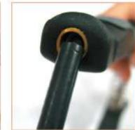
Housing Reformer for easy installation of ferrules.
