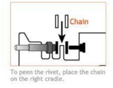
Always place the chain on the left cradle for breaking or assembly.
