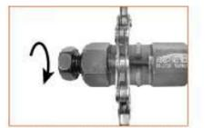
To hold the chain by tightening the bolt. Make sure the bolt is locked accurately.
