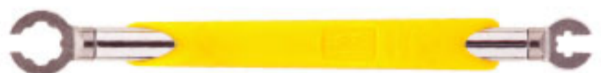
TB-5518 Spoke wrench For both Mavic® 9 mm threaded eyelets and Mavic® 6 splines of integrated nipples with 5.65 mm outside diameter and 7 mm thread nipple.
